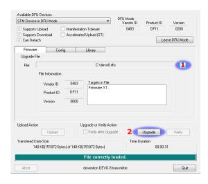
Plug the transmitter into the PC via USB, and turn on the transmitter while holding 'EXT' to enter programming mode. On the Devo12, this is done by holding the trainer switch instead.
