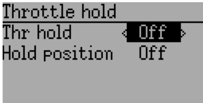
The throttle-hold page is used to enable/disable the throttle-hold capability. Specifying 'Hold position' defines the throttle value when the Throttle-hold switch is set. Hold position can be set from -200 to 200.
