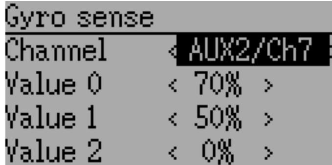
The gyro-sensitivity page enables configuring up-to 3 sensitivity values for the gyro as well as which channel to use for sending the gyro value. Acceptable values range from 0 to 100%.
