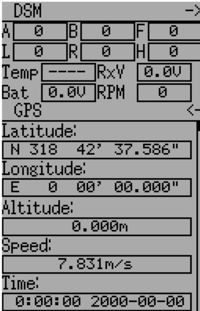
The following fields are available in DSM2 Telemetry. Note that a dedicated telemetry module and additional sensors are needed to capture this data
