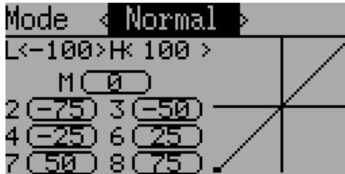
The pitch curve allows defining a piece-wise linear curve for the collective/pitch channel. Different curves can be selected for each flight-mode as well as for throttle-hold. Each point value can be enabled to be interpolated from the points surrounding it.
