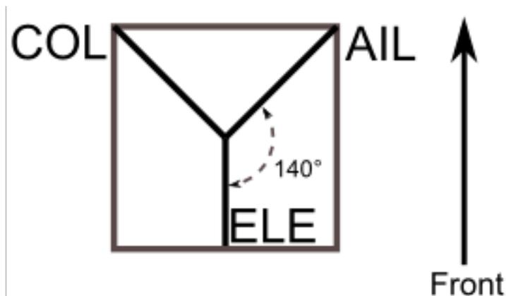
**140 (3 Servo):** Fundamentally, the servo operations of 140° swash-plates are almost the same as 120° swash-plates. However, the servo arrangement for elevator operation differs. 140° swash-plate CCPM offers smoother operation of the combined servos and an equal cyclic rate all around. On a 120° setup, the left/right cyclic is slightly faster than the fore/aft cyclic.
