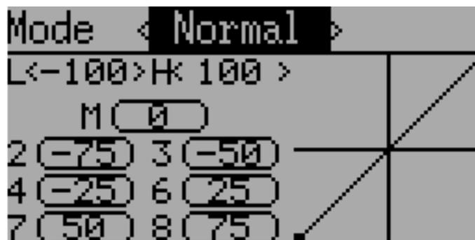
The throttle curve page allows defining a piece-wise linear curve for the throttle channel. Different curves can be selected for each flight-mode. Each point value can be enabled to be interpolated from the points surrounding it.
