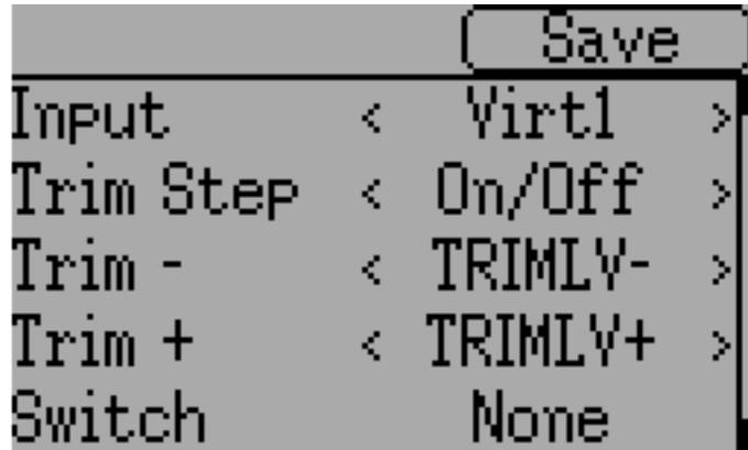
Next set the 'Trim Step' field to 'Momentary', 'Toggle', 'On/Off' or '3 Pos'. This is done by pressing the left-arrow on the 'Trim Step' spin-box until the value is less-than 0.1 Second select the 'Input' to be the virtual channel to convert to a switch (we'll use 'Virt1')
