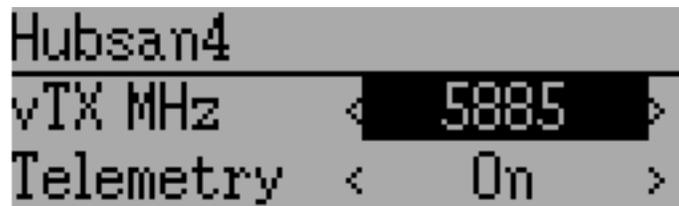
The Hubsan4 protocol supports up to 13 channels, regular format only supports auto-binding. The fixed ID can be used, but does not prevent auto-binding during power-on. The 1 st 4 channels represent Aileron, Elevator, Throttle, and Rudder. Additional channels control the quadcopter special functions:
