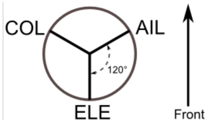
**120 (3 Servo):** Servos are placed around the swash-plate at 120° intervals. With Aileron input, the aileron and pitch servos tilt the swash-plate left and right; with Elevator input, the three servos tilt the swash-plate fore and aft; with Pitch input, all three servos raise the swash-plate up and down. Servos working in unison dramatically increases the torque available as well as the precision and centering.
