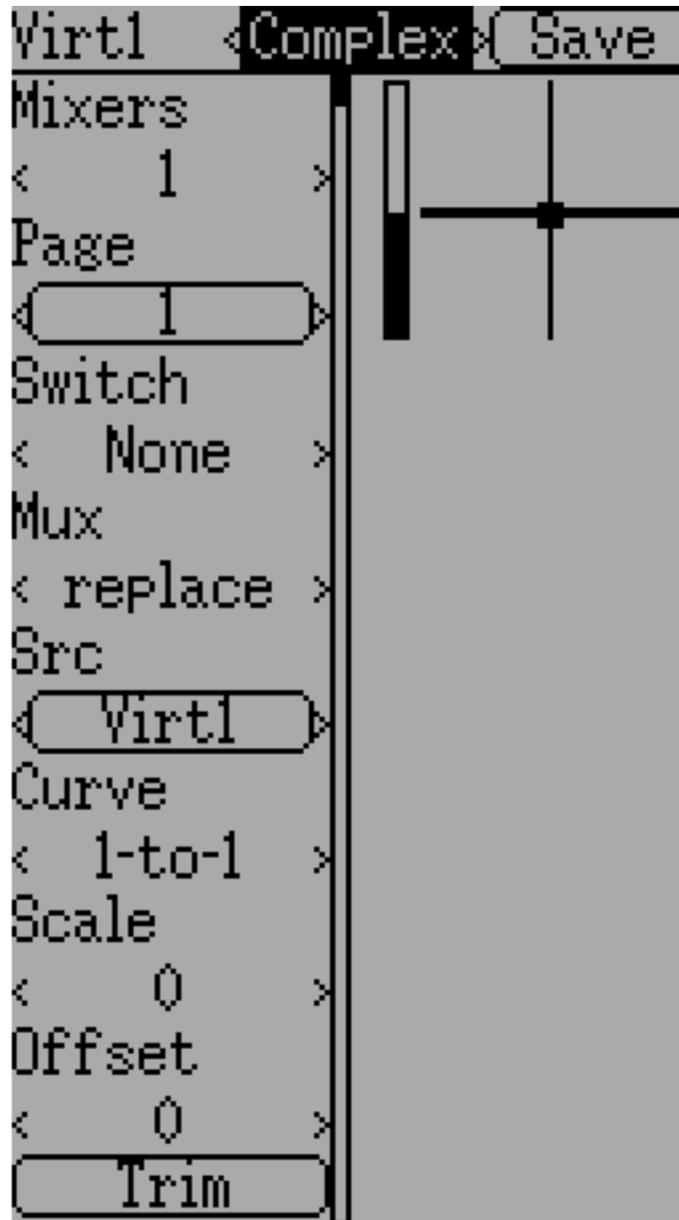
Now go to the 'Mixer' page, and enter the configuration for the specified Virtual Channel (Virt1 in our example)
