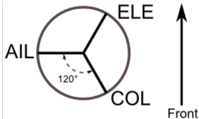
**120X (3 Servo):** Same as the above layout except servos are shifted 150°. With Aileron input, the three servos tilt the swash-plate left and right; with Elevator input, the elevator and pitch servos tilt the swash-plate fore and aft; with Pitch input, all three servos raise the swash-plate up and down.
