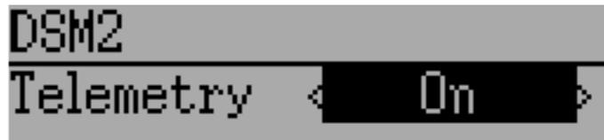
The DSM2 protocol also supports enabling/disabling the telemetry capability. This option is accessed by pressing the Protocol spin-box when DSM2 is shown.
