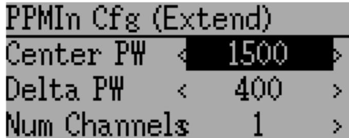
Deviation has the ability to use PPM input signals from an external source (such as an FPV setup). To configure this mode, set the PPM In mode to ‘Extend’ in section *Model setup (Std & Adv GUI)*.
