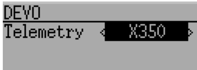
The DEVO protocol also supports enabling/disabling the telemetry capability. This option is accessed by pressing the Protocol spin-box when DEVO is shown. The options are Std (standard format), X350 (Walkera QR-X350 format), and Off.
