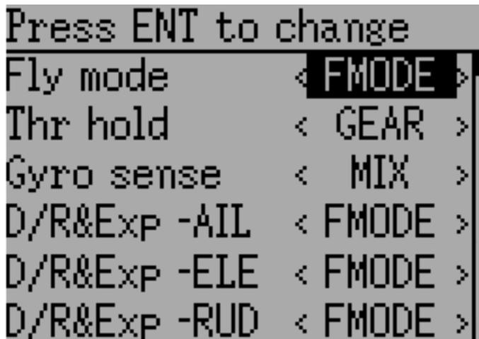
The switch assignment page enables configuring which switches to use for each capability in the standard-GUI. The same switch may be assigned to multiple capabilities.
