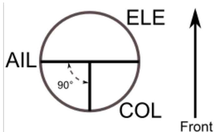
**90 (3 Servo):** With Aileron input, the aileron and pitch servos tilt the swash-plate left and right; with elevator input, the servos tilt the swash-plate fore and aft; with Pitch input, all three servos raise the swash-plate up and down. Most commonly used for electronic helicopters.
