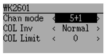
The WK2601 protocol also supports additional options. These are accessed by pressing the Protocol spin-box when Wk2601 is shown:
