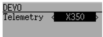
The DEVO protocol also supports enabling/disabling the telemetry capability. This option is accessed by pressing the Protocol spin-box when DEVO is shown. The options are Std (standard format), X350 (Walkera QR-X350 format), and Off.
