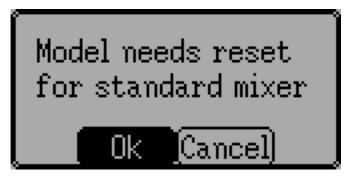
**Mixer GUI**: Defines which graphical user interface (GUI) to use for this model. The 'Advanced' GUI is the default for Deviation. The 'Standard' GUI is only available for Helicopter models and more closely resembles the stock GUI.
