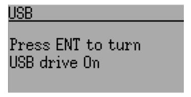
The USB page can be accessed by selecting 'USB' from the main menu. USB mode can then be toggled on/off to enable access to the transmitter's file-system from a USB equipped computer. In this mode the file system of Deviation is accessible as a mass storage device. This will allow you to move files back and forth between the Deviation file-system and a PC. All configuration files are accessible in this mode.
