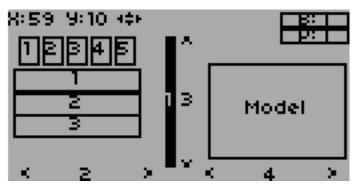
Pressing and holding the ENT button from the model configuration page will switch to the object position screen. Each of the visual objects can be selected using the UP/DN buttons. Pressing ENT again will allow moving the placement of the selected object. The UP/DN/L/R buttons will move the selected object on the screen. Press EXT once to exit move mode, and again to go back to the main page config menu.
