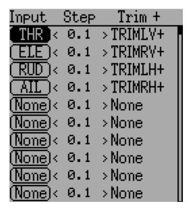
The trim page allows assigning the trim buttons and trim step, as well as configuring buttons to work as virtual inputs (see *Using a Trim as a Virtual Switch*). It is accessed from the main menu via "Model menu" followed by "Trims".
