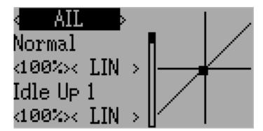
The dual-rate and expo page allows configuration of curves for the Aileron, Rudder, and Elevator channels. Up-to 3 rates can be configured for each channel, and either a scaled-linear or exponential curve can be
