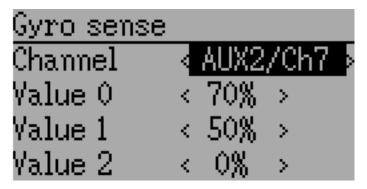
The gyro-sensitivity page enables configuring up-to 3 sensitivity values for the gyro as well as which channel to use for sending the gyro value. Acceptable values range from 0 to 100 %.
