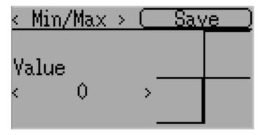
For the Min/Max, Zero/Max, >0, <0, and ABSVAL, the controls allow setting the transition point along the x-axis. A value of '0' will be symmetric around the y-axis, positive or negative values will move the center point accordingly
