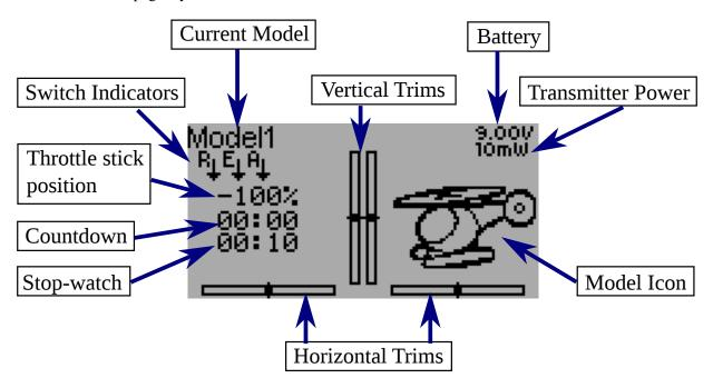
**Current Model**: The name of the current model. Clicking the label will open up the Model Load page. The model is configured from section *Model setup (Std & Adv GUI)*.
