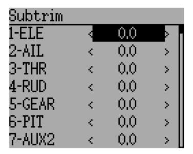
The sub-trim adjust page allows setting the zero-point of the servos for each channel. This is equivalent to the 'Subtrim' setting on the Channel Configuration sub-page of the Mixer menu when using the Advanced GUI (see *Channel configuration*). Acceptable values range from -50 to +50 in 0.1 increments.
