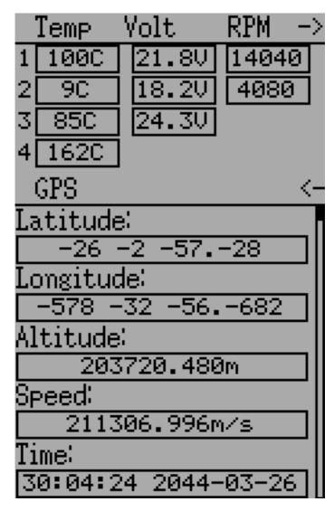
Certain protocols have the ability to transmit telemetry data back to the transmitter during use. Telemetry data may include, but is not restricted to, temperature readings, various voltage readings, motor or engine rpm, as well as GPS related information.
