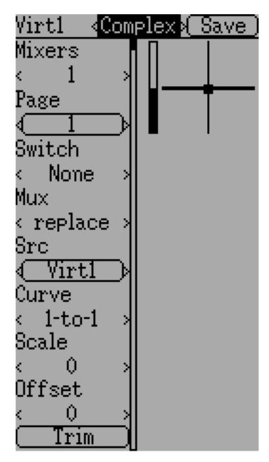
Now go to the "Mixer" page, and enter the configuration for the specified Virtual Channel (Virt1 in our example)
