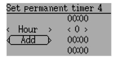
The 'permanent' timers are similar to an odometer and have their values saved in the model.ini file. They will maintain their previous value when powering up the transmitter. You can set the timer by using the "Set to" button and reset by pressing the "Reset" button.
