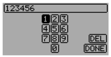
**Fixed ID**: The Fixed ID sets a unique code to ensure that the transmitter will only bind to a specific model. This is useful to ensure that the transmitter is not accidentally bound to the wrong model.
