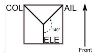
**140** (**3 Servo**): Fundamentally, the servo operations of 140° swash-plates are almost the same as 120° swash-plates. However, the servo arrangement for elevator operation differs. 140° swash-plate CCPM offers smoother operation of the combined servos and an equal cyclic rate all around. On a 120° setup, the left/right cyclic is slightly faster than the fore/aft cyclic.
