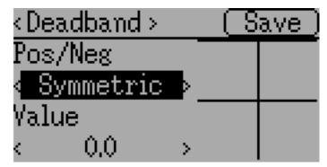
For the Deadband curve, the controls allow independently configuring the deadband width for values greaterthan or less-than zero.
