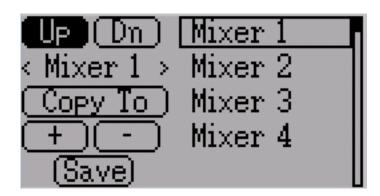
Select the respective mixer and use the up/down buttons to move the order of the selected mixer. Note that the mixer name represents its position when the reorder dialog was opened. If the dialog is closed and reopened, all mixers will be shown as numbered sequentially.
