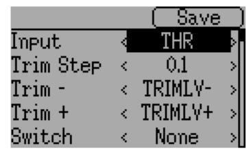
The trim-step defines how sensitive the trims are to input. The maximum number of trim steps is  $\pm$ 100. So a step size of 0.1 will allow a full  $\pm$ 10% of trim adjustment on the servo.
