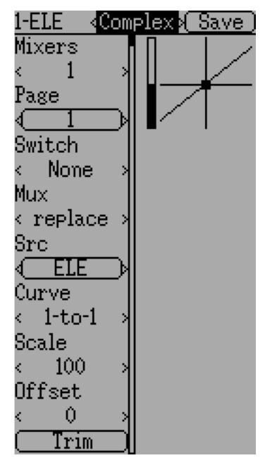
The Complex mix type unlocks the full power of the mixer system. For a given channel, any number of mixers can be applied to affect the final result. Each mixer is applied based on whether the specified switch is active, and can either replace, add to, or multiply to the previous mixers for this channel. Using this system
