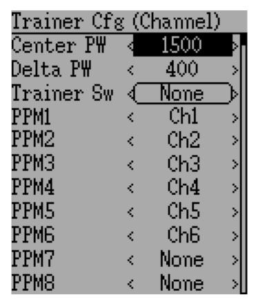
**Channel**: In channel mode, each input channel is mapped to an output channel on the instructor's transmitter. In this mode, the student's transmitter should do all necessary mixing to control the model. Care must be taken to ensure that the instructor and student transmitters are configured identically, otherwise, the model may not react well when switching between instructor and student control.
