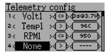
The telemetry configuration page allows specifying alarms when specific telemetry events occur.
