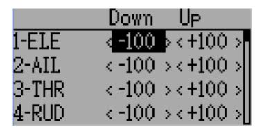
The servo-travel adjust page configures the maximum positive/negative travel of each servo. This is equivalent to the 'Scale+' and 'Scale-' settings on the Channel Configuration sub-page of the Mixer menu when using the Advanced GUI (see *Channel configuration*). Acceptable values for Down are from -175 to -1 and Up values range from +1 to +175. The default values are -100 and +100 respectively.
