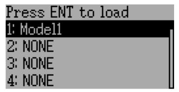
**File**: The File spin-box allows loading a new model, copying the existing model to a new location, resetting the current model to the default (all configuration is lost), and loading templates (see *Predefined Model Templates*). Note that changing models may result in a safety message being displayed (see *Safety System*).
