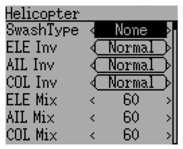
**Model Type**: Set the model-type available options are Heli, Plane and Multi. Helicopter models have an additional configuration page that can be accessed by clicking the Model type. The options for SwashType are identical to the ones in *Swash Configuration*.
