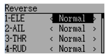
The servo reverse page allows quickly setting each channel to work in either normal or reversed mode. These settings are equivalent to the 'Reverse' setting on the Channel Configuration sub-page of the Mixer menu when using the Advanced GUI (see section *Channel configuration*)
