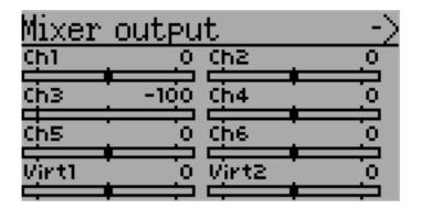
The channel monitor screen allows the user to see the values of each channel as output by the transmitter. Channels without mixers will not be displayed. Channel output displayed is the value based on minimum / maximum values as well as scaling.
