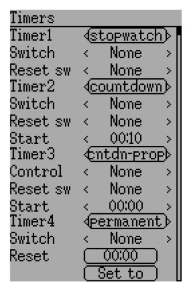
The timer page defines up to 4 available timers. Timers can count either up or down, and can be enabled either manually from the main screen or by an input trigger (stick or switch).
