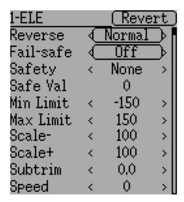
The Channel configuration provides the ability to configure the final channel outputs. Capabilities such as channel reverse and fail-safe values are applied here. Also available are controls for end-points, scaling, sub-trim, and a safety switch (which could be used to ensure that a motor cannot spin-up while working on a model)
