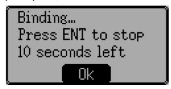
**Bind/Re-Init**: Depending on the protocol and Fixed-ID setting, the transmitter may bind with the model on start-up, or may need to be manually bound once. See *Protocols* for more on specific protocols. If the protocol does not support binding, the button will show 'Re-Init', which can be used to switch protocols without power-cycling the transmitter.
