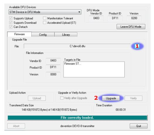
Unzip the firmware file that you downloaded earlier. Plug the transmitter into the PC via USB, and turn on the transmitter while holding 'EXT' to enter programming mode.
